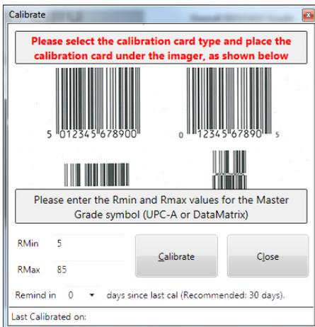
Select the linear barcode, and make sure the Rmin and Rmax values match those on your calibration card. Set the calibration reminder to 15 days, and then click on the calibrate button. The calibration will take about 5 seconds and then the successful window will appear. Press **OK**, and then close the window.
