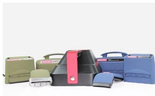
After you receive your verifier back from the calibration service it is important that you carry out the user calibration before using. This ensures that its reflectance measurements are aligned with the reference standard values on the calibration card.
